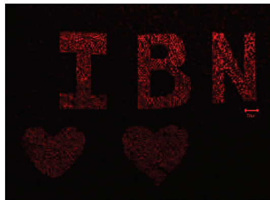
Figure 6. Photograph of a photoluminescent pattern generated by two-photon laser writing on a solid substrate coated with CdSe@CdS QDs with excess sulfur. Scale bar represented 20 \mu\text{m} .
